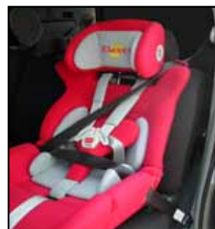
Fix the seat belt of buckle side of your car through the belt holder.
