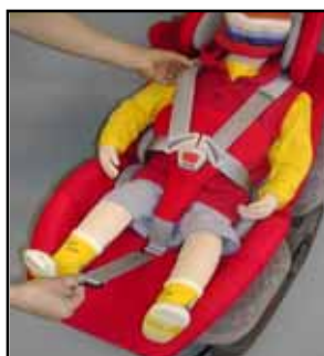
pulling out the belt of the hand-operated belt adjuster to shorten the shoulder belt
