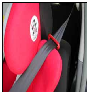
Put the seat belt of your car through the belt holder of the back.
